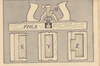
If the mortise is wider than the width of the cutter being used, adjust the fence for the new cut and proceed as before, making the first and successive cuts as instructed.
