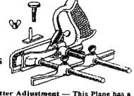
Cutter Adjustment — This Plane has a handy Cutter Adjustment, conveniently located to obtain the proper depth of cut. Always loosen the Wing Nut slightly on Main Stock before adjusting Cutter and then tighten securely after the Cutter is properly set.
